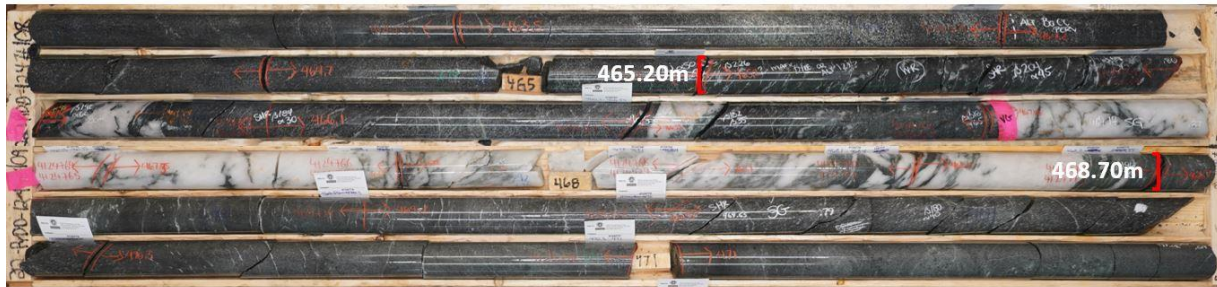
R5 VEIN: 22RDD124, 465.20m-468.70m (assays pending): Biotite altered diorite with up to 5% sulphide, quartz calcite veinlets, quartz-sulphide veining with visible gold
