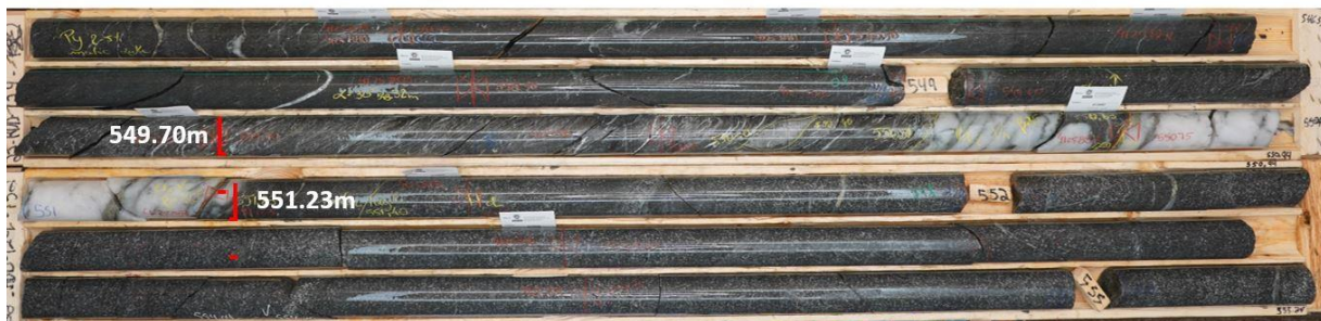
NEW DISCOVERY: 22RDD129, 549.70m-551.23m (assays pending): Strongly strained biotite chlorite altered diorite with up to 5% sulphide, quartz-sulphide-telluride veining
