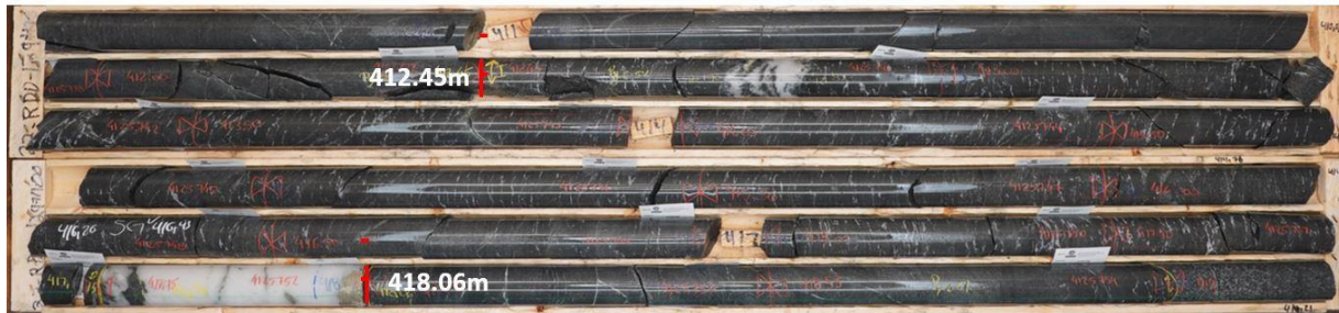
NEW DISCOVERY: 22RDD129, 412.45m-418.06m (assays pending): Biotite-chlorite altered diorite with up to 5% sulphide, strong quartz calcite veinlets, quartz-sulphide veining
